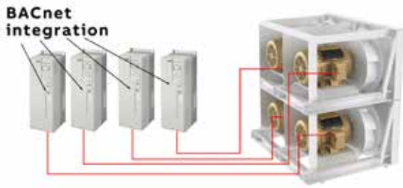
Figure 3: One VSD per motor fan array
